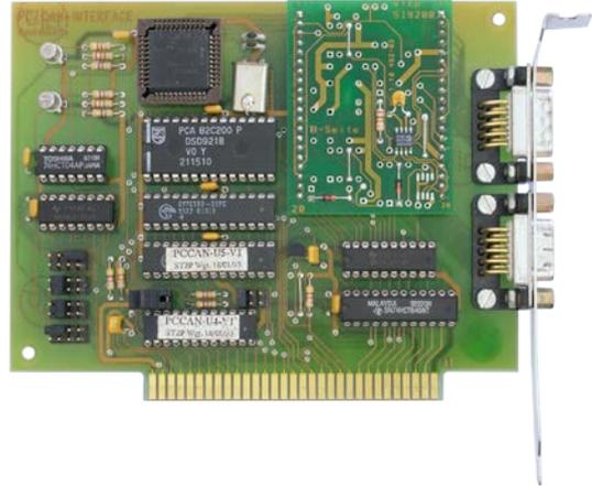
Figure 2: First PC CAN interface board with ISA bus hosting the Philips 82C200 (BasicCAN) and already the Intel 82527 (FullCAN) CAN controller chips (Source: STZP / HMS)
