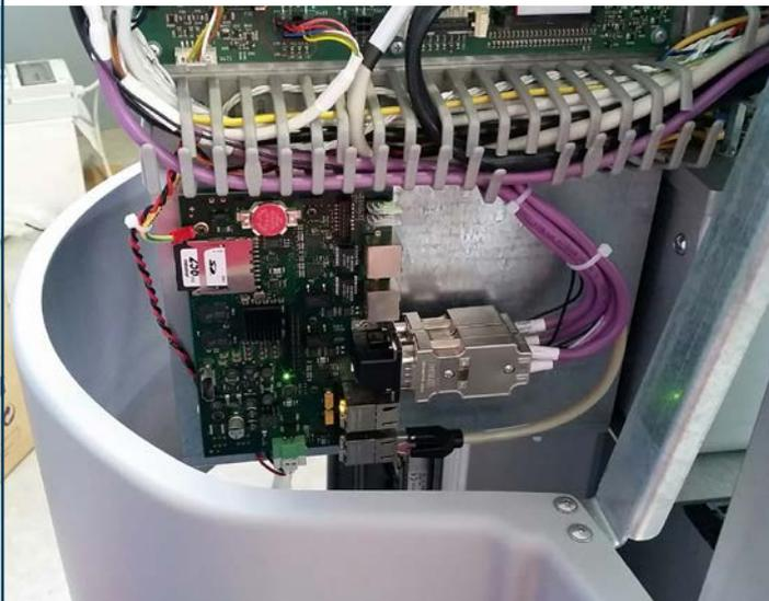
**On the inside.** The ECON100 (without the blue housing) embedded into the Giotto Class Digital Breast Tomosynthesis machine.
