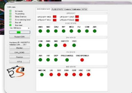
Control panel showing the fuses in the car.
