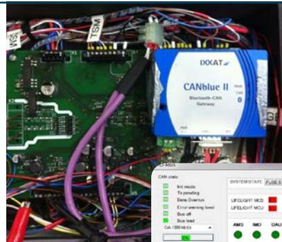
The Ixxat CANblue II sends data from the racing car to a diagnostics system on a PC in the pit stop.
