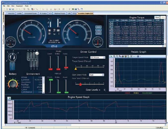
Example of a test dashboard in the LABCAR user interface.
