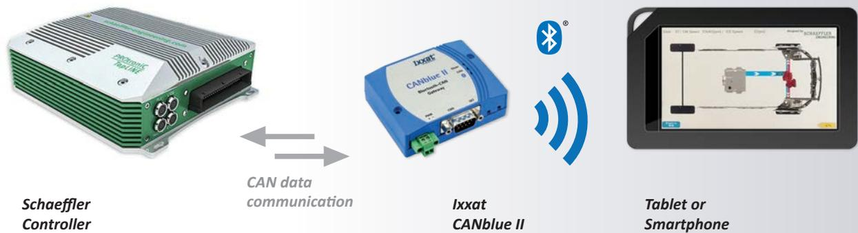
*CANblue II connects ECU of testvehicles via Bluetooth with Smartphones or Tablet PCs.*
