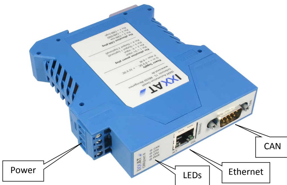
Figure 3-1 Connectors and displays of the CAN@net II/Generic
