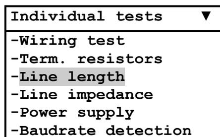
When the CAN network is switched off, the test instructions appear. Error messages are explained in section 6. When the test instructions are executed, start the test with the **OK** key.
