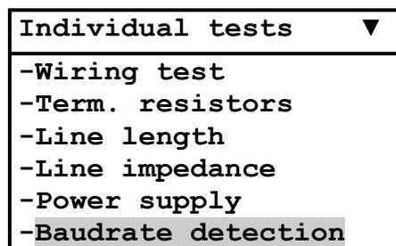
During the measurement, a message appears. After the measurement, the test result appears. Error messages are explained in section 6.
