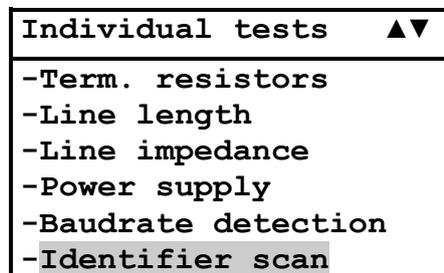
During the measurement, first the baudrate is detected and the relevant message appears. Then the scan for identifiers is carried out and a further message appears.
