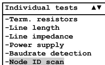
During the measurement, first the baudrate is detected and the relevant message appears. Then the node ID scan is carried out and a further message appears.
