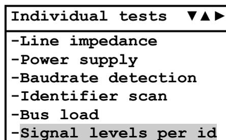
During the measurement, the baudrate is detected and the relevant message appears. Then the scan for identifiers is carried out and a second message appears. The signal levels are measured and a third message appears.
