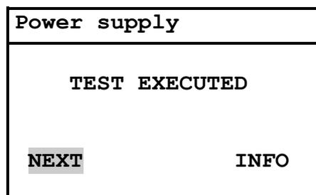
Start the next test with the virtual key **NEXT**. First, however, we want to look at the test results with the virtual key **INFO**. For this, change to the virtual key **INFO** with the key **RIGHT**. This appears in black with white lettering. Confirm the selection with **OK**.
