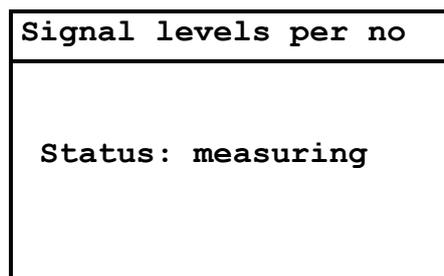
After the measurement the test result appears. The beginning of the list is shown here. Scroll through the list with the keys **UP** and **DOWN**.
