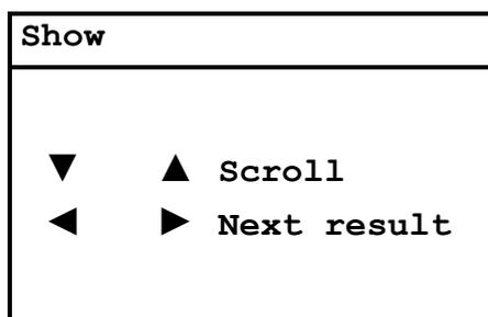
If menu items **Results** and **Show** are selected immediately after switching on the CANcheck and the key **LEFT** is pressed, the result **No valid results** is shown.
