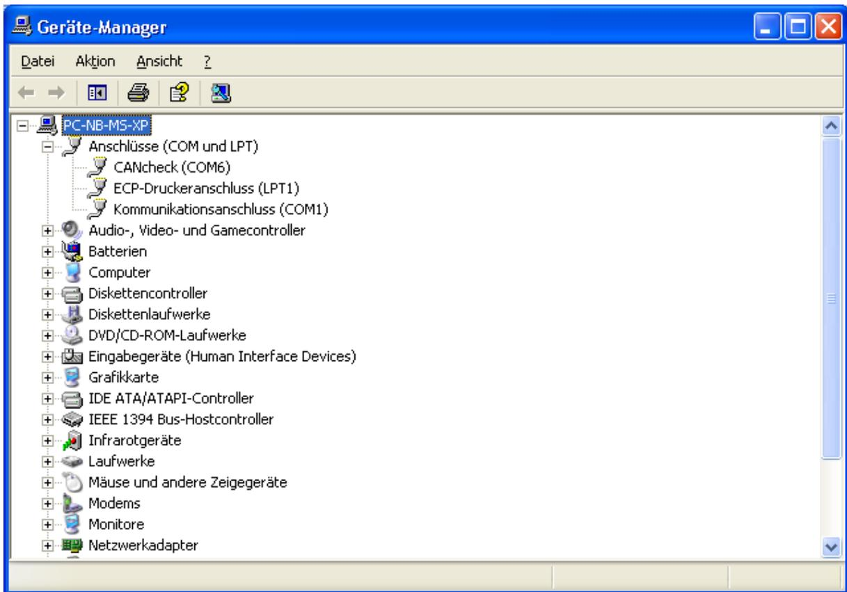
To **test** the connection between the CANcheck and the PC, start a terminal program (e.g. Hyperterminal) on your PC.
