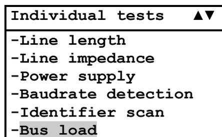
During the measurement, the baudrate is detected and the relevant message appears. Then the bus load is measured and the interim results are shown “online”.
