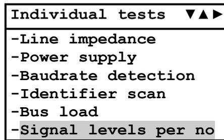
During the measurement, the baudrate is detected and the relevant message appears. Then the scan for node IDs is carried out and a second message appears. The signal levels are measured and a third message appears.
