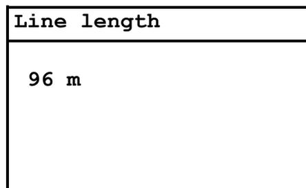
Continue the tests of the line parameters by returning to the higher order menu with the **ESC** key. Start the next test with the virtual key **NEXT** and the **OK** key. Now the termination resistor is measured. The test instructions are the same as for the wiring test.
